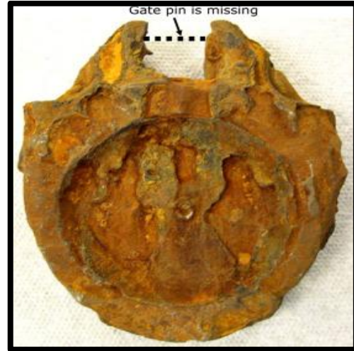
Figure 4. General (uniform) corrosion Source: Handbook of Environmental Degradation of Materials (3rd Edition), 2018
