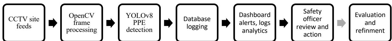
Figure 2 System workflow of P.P.Eye-TRACK from CCTV input to dashboard-based safety action and evaluation
